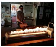
it is designed to dramatically demonstrate how sound waves are propagated through the air, or in this case a flammable gas. Once the tube became connected to the laboratory gas supply the gas emerging through the holes along the length -field view of sections of the night sky. of the tube could be lit, resulting in a neat row of small through the gas inside.
