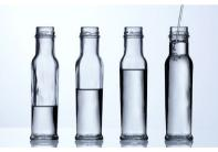
if you tap the side of the bottle with a wooden stick or mallet. The sound frequency/pitch gets <u>lower</u> as the amount of water in the bottle increases.
