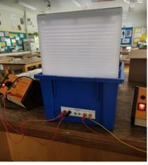
provide perfectly stationary images of the pattern of waves and the large front facing screen makes this ripple tank ideal for classroom demonstrations. There is also an extensive range of accessories, including three dippers and a selection of barrier shapes and lenses.
