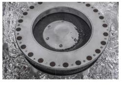
So far the samples have been analysed using a number of different techniques - the dust was put in a scanning electron microscope, and probed via infrared spectroscopy, X-ray diffraction and chemical element analysis. X-ray computed tomography (CT) was used to make 3D models of particles and look inside them. One of the key findings is the presence of that carbon. Lots of it. Close to 5% by weight.
